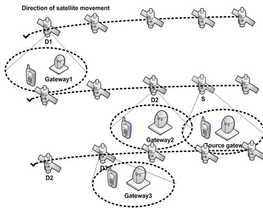
Figure 1. Multicasting in LEO satellite constellation.
