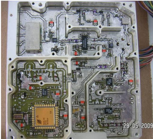
Figure 2. Uncovered on-board transceiver EM
