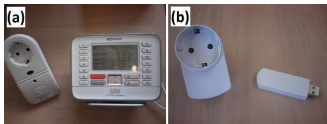
Figure 2: Smart meters (a) EcoManager (Current Cost) and (b) Plugwise
