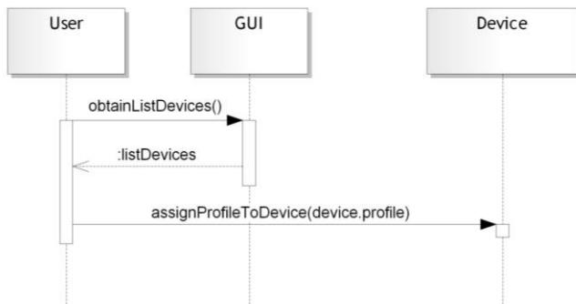
Figure 6: Sequence diagram: Election of an energy profile
