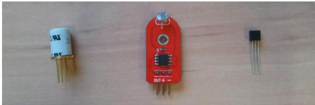
Figure 3: Carbon monoxide (CO), luminosity and temperature sensors
