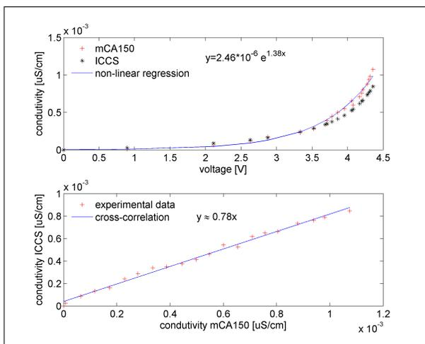
Figure 8. Calibration curves and comparison of measurements of the electrical conductivity from experimental solutions obtained with the intelligent and customized sensor with cell constant of  $0.255\text{ cm}^{-1}$ .
