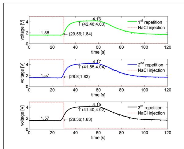
Figure 11. Transients and transport delay times of the sprayer with the conductivity sensor assembled in an actual spraying system with water-NaCl solution flow of  $16\text{ l/min}$  and pressure equal to  $200\text{ kPa}$ .
