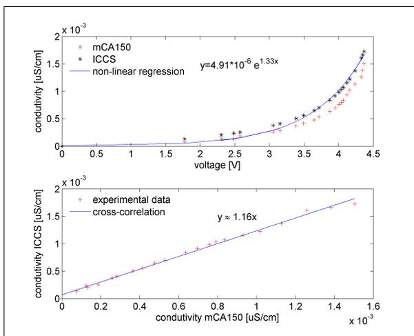
Figure 9. Calibration curves and comparison of measurements of the electrical conductivity from experimental solutions obtained with the intelligent and customized sensor with cell constant of  $0.500\text{ cm}^{-1}$ .
