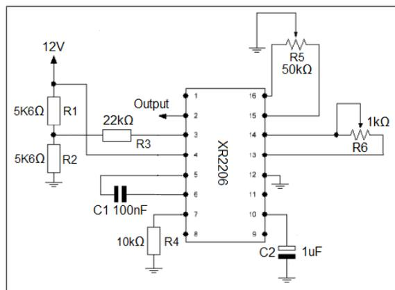
Figure 4. Circuit for the excitation signal generator.
