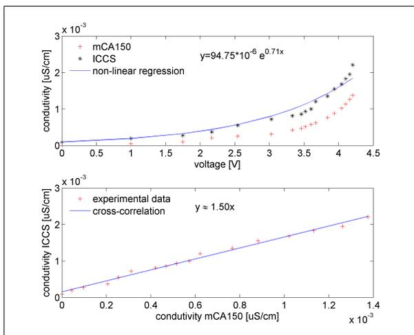
Figure 10. Calibration curves and comparison of measurements of the electrical conductivity from experimental solutions obtained with the intelligent and customized sensor with cell constant of  $0.764\text{ cm}^{-1}$ .
