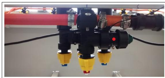
Figure 6. Instrumental arrangement for validation of the intelligent sensor to measure response time of a direct injection sprayer with TeeJet® QJS Multiple Nozzle Bodies e-ChemSaver.
