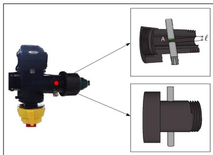
Figure 5. Details of the smart sensor customized to measure the response time of a system of direct injection of pesticides.
