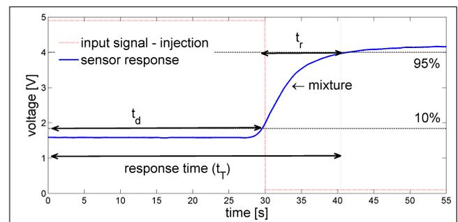
Figure 1. The delay time  $t_d$ , rise time  $t_r$  and response time  $t_T$  involved in a typical injection system as defined in [24]. The red line indicates the behavior in time of the concentrated mixture (water-NaCl) as an injection input.
