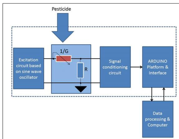
Figure 2. Block diagram of the customized intelligent sensor for response time measurements in spraying systems based on direct injection of pesticides.
