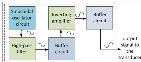
Figure 3. Block diagram of the excitation circuitry.
