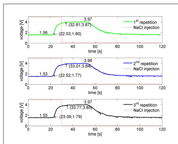
Figure 12. Transients and the transport delay times obtained with the intelligent conductivity sensor assembled in an actual spraying system with water-NaCl solution flow of  $23\text{ l/min}$  and pressure equal to  $400\text{ kPa}$ .
