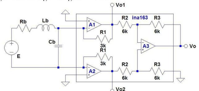
Figure 6: Signal conditioning for Flux mode magnetometer
