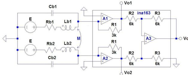
Figure 10: Flux mode differential magnetometer structure
