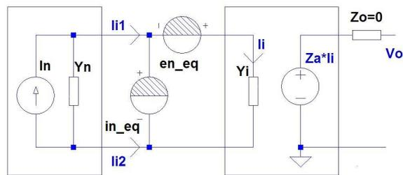
Figure 4: Equivalent electrical model of the Flux mode magnetometer.  $Z_a$  is the amplifier transimpedance and  $Y_i$  is the input admittance, which has to be as large as possible.
