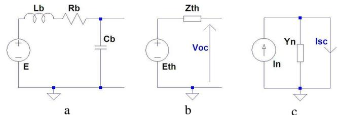
Figure 1: Electrical equivalent circuit of a search coil (a) operating in Lenz mode (b) or Flux mode (c). In Lenz mode the magnetic flux is related to the open circuit voltage  $V_{oc}$  whereas in Flux mode, the flux density is related to the short circuit current  $I_{sc}$ .
