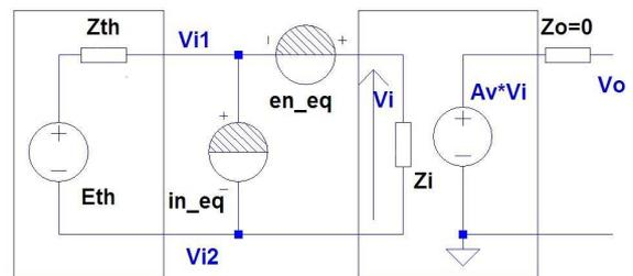
Figure 3: Equivalent electrical model of the Lenz mode magnetometer.  $A_v$  is the voltage Gain and  $Z_i$  the input impedance, which has to be as large as possible.
