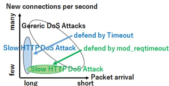
Figure 5. Conceptual diagram of the range to be defended
