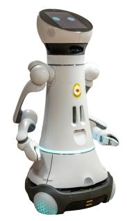
Figure 1. The assistive robot Care-O-Bot 4 configured with two arms and spherical hip and head joints.
