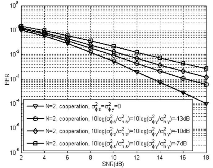
Fig. 3. BER performance of  $N = 2$  cooperative distributed relay networks under certain/uncertain channel conditions using both imperfect channel vectors  $(\bar{\mathbf{h}}_s, \bar{\mathbf{h}}_y)$ .
