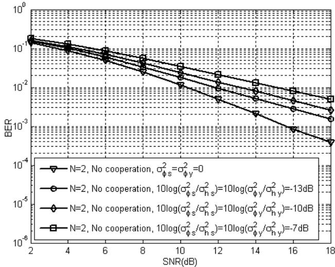
Fig. 5. BER performance of  $N = 2$  noncooperative distributed relay networks under certain/uncertain channel conditions using both imperfect channel vectors  $(\hat{\mathbf{h}}_s, \mathbf{h}_y)$ .
