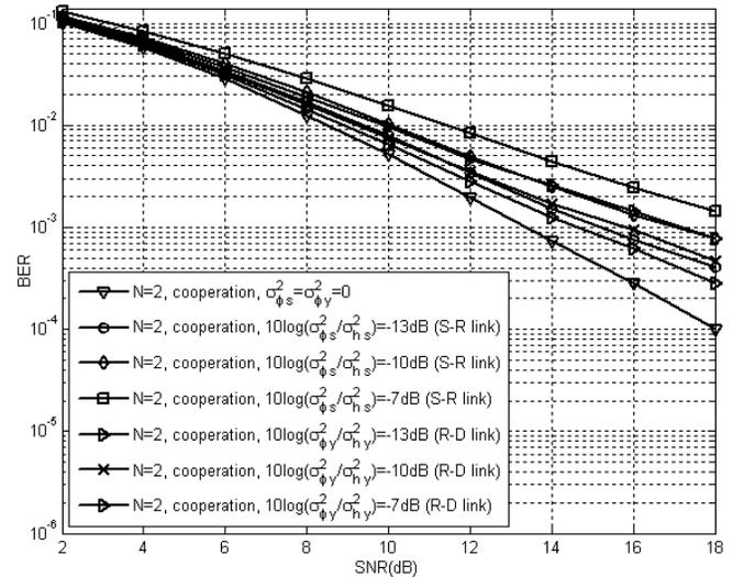
Fig. 4. BER performance of  $N = 2$  cooperative distributed relay networks under the cases of  $(\bar{\mathbf{h}}_s, \mathbf{h}_y)$  or  $(\mathbf{h}_s, \bar{\mathbf{h}}_y)$ .
