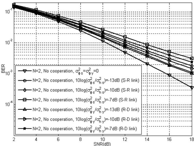
Fig. 6. BER performance of  $N = 2$  noncooperative distributed relay networks under the cases of  $(\hat{\mathbf{h}}_s, \mathbf{h}_y)$  or  $(\mathbf{h}_s, \hat{\mathbf{h}}_y)$ .
