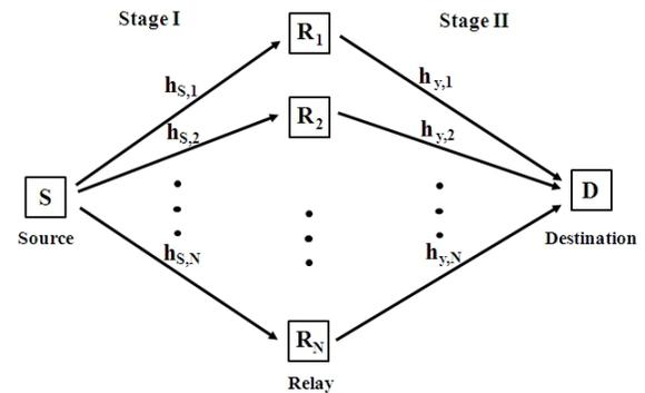
Fig. 1. Wireless relay network with one-source-one-destination pair and  $N$  relay nodes under no channel uncertainty ( $\mathbf{h}_s, \mathbf{h}_y$ ).
