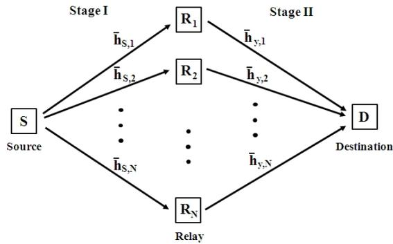
Fig. 2. Wireless relay network with one-source-one-destination pair and  $N$  relay nodes under channel uncertainty for both source-relay links and relay-destination links ( $\bar{\mathbf{h}}_s$ ,  $\bar{\mathbf{h}}_y$ ).
