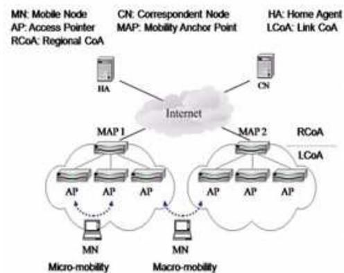
Figure 1. Hierarchical Mobile IPv6
