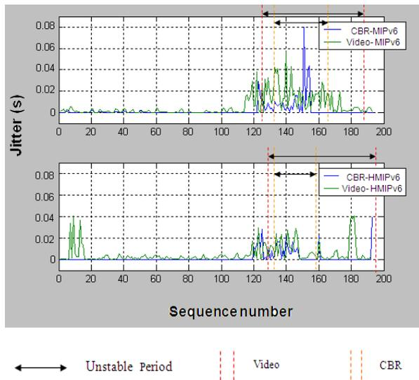
Figure 7. Jitter vs. Sequence number generated
