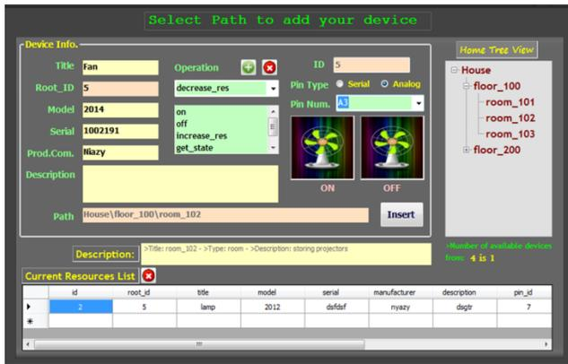
Figure 3. Locating and configuring a fan device at logical path 'floor\_100\room\_102.'
