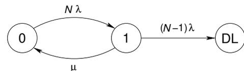
Figure 1. Reliability model for a RAID-5 array.
