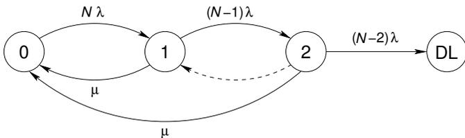
Figure 2. Reliability model for a RAID-6 array.
