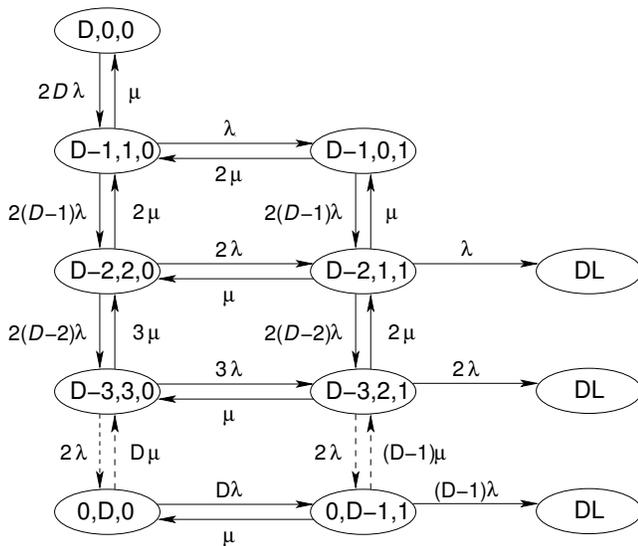
Figure 3. Reliability model for a RAID-51 array.
