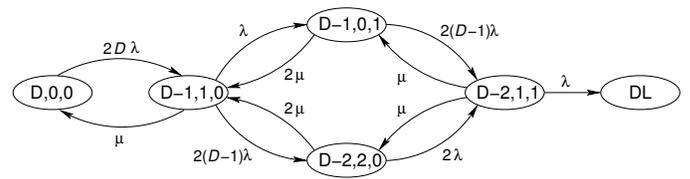
Figure 4. Shortest-path reliability model for a RAID-51 array.
