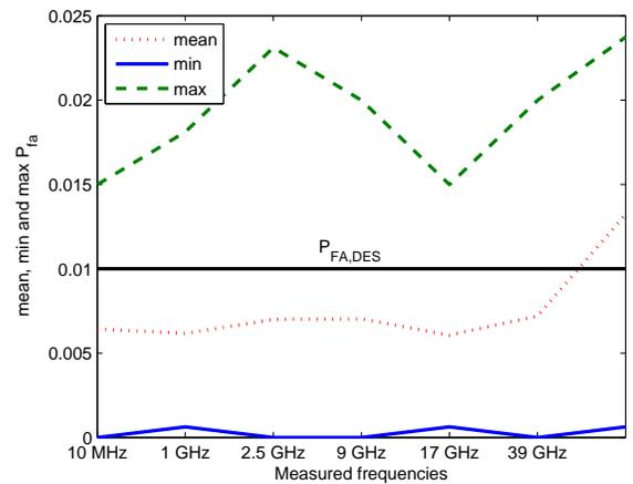
Figure 9. Mean  $P_{FA}$ , min  $P_{FA}$  and max  $P_{FA}$  values for different frequency areas.  $N=1601$ . Measured noise.
