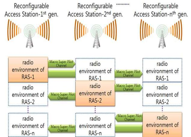
Figure 4. Access method of macro-band SPC between RASs
