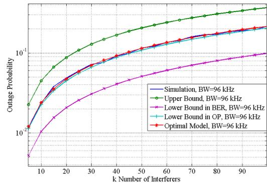
Figure 8: OP as function of  $k$  interferers, for  $BW = 96$  kHz.
