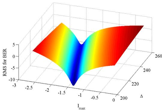
Figure 5: RMS for BER vs the couple  $(\Delta, I_{max})$ , for  $I_{min} = -90$  dB,  $k = 20$  interferers and  $BW=12$  kHz.
