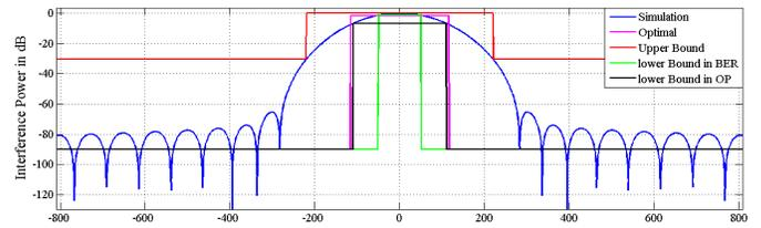
Figure 2: Behavior of interference vs frequency difference  $\delta_f$ .
