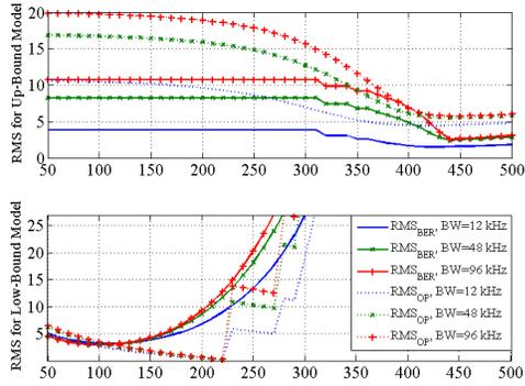
Figure 4: RMS for BER and OP vs  $\Delta$ , for  $k = 100$ , different bandwidth length.
