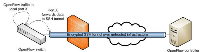
Figure 3. Secure SSH tunnel transporting the OpenFlow data.
