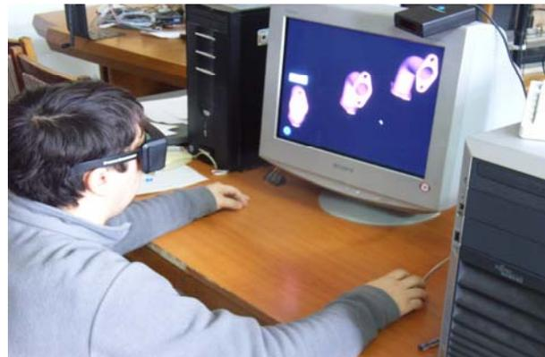
Figure 2. The subject selecting a 3D model using 3D display active stereoscopic visualization system
