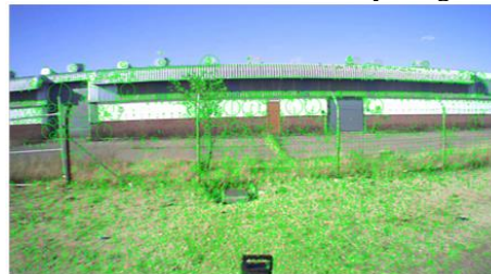
Figure 5. Detecting the image feature using SIFT algorithm.
