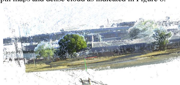
Figure 8. Denser point of cloud with multiview stereo.
