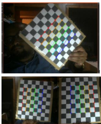
Figure 4. Black and white test match on a chessboard.
