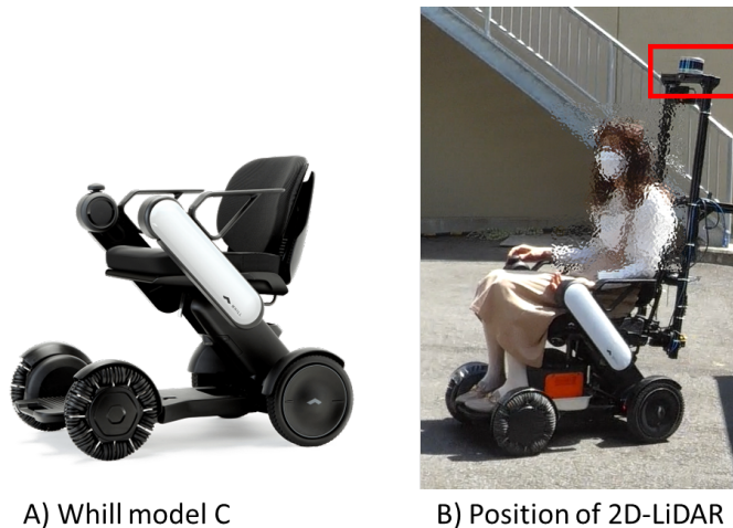
Figure 1. PM (A) and 2D-LiDAR position (B).
