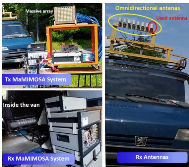
Figure 2. Tx-Rx antenna systems.
