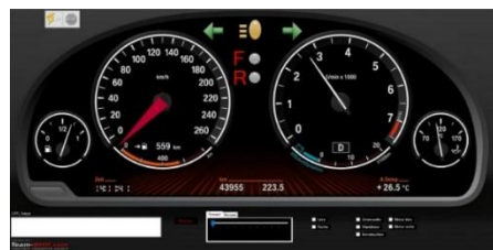
Figure 15. Interface to control the CAN-Demonstrators inside the CANoe-Tool
