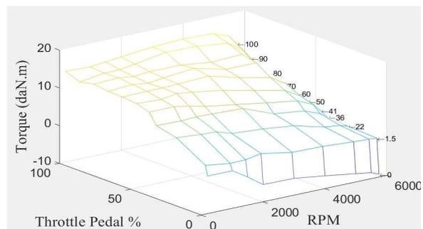
Figure 1. Engine Torque cartography used in vehicle model
