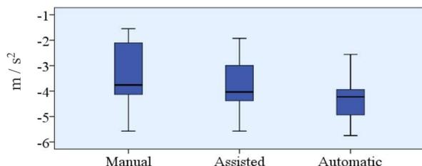
Figure 9. Maximum deceleration in braking in Section A
