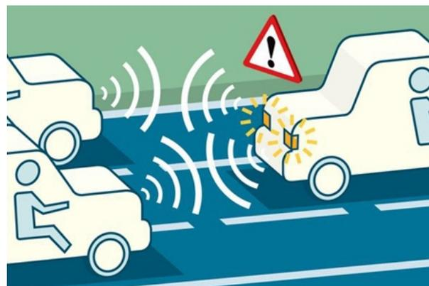
Figure 1. Visible Light Communication for V2V information exchange.
