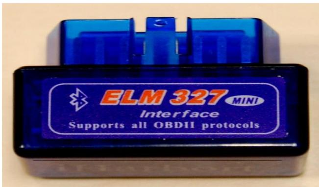
Figure 4: ELM 327 OBDII device
