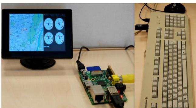
Figure 3: Prototype of Modularized webinos, running on a Raspberry Pi Hardware and showcasing IVI-system view connected to an OBD simulator
