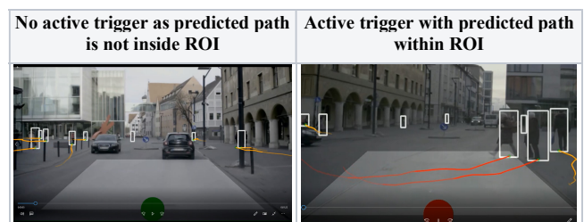
Figure 7. Trigger examples with trajectory prediction
