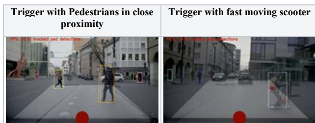
Figure 5. Trigger examples with pedestrian detections
