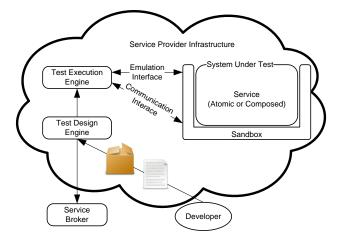
Figure 4. Test Environment for IoT enabled Composite Service
