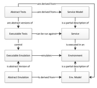
Figure 1. Extended model based testing approach
