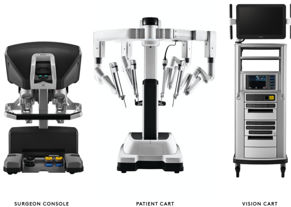
Figure 3. The da Vinci surgical system [21].
