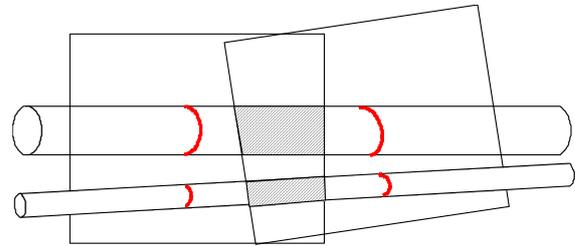
Figure 13. Connection of two point cloud data sets.
