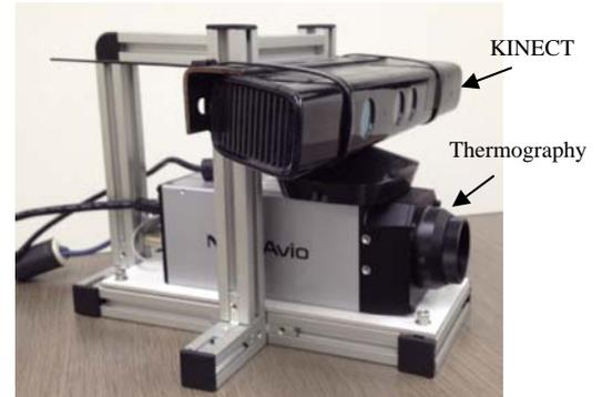
Figure 1. Measurement system.
