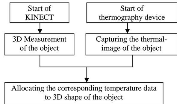
Figure 2. Measurement procedure.
