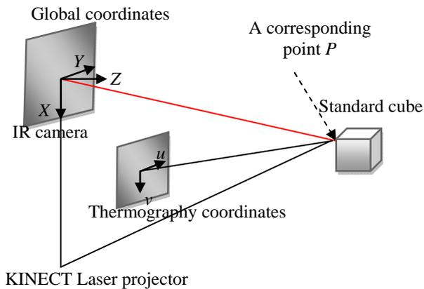
Figure 3. Calibration setup.
