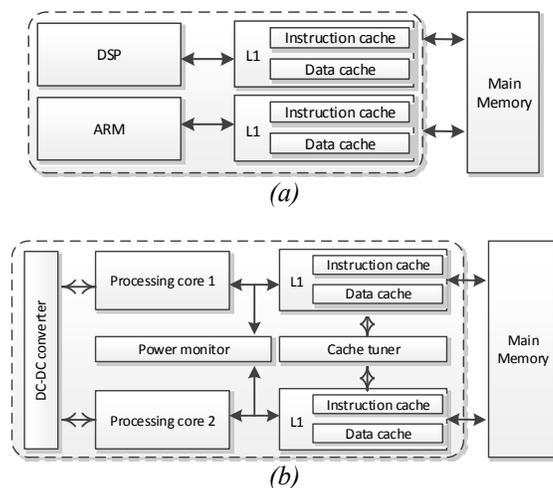
Figure 1. Layout of a sample (a) heterogeneous dual-core system and (b) configurable homogeneous dual-core system
