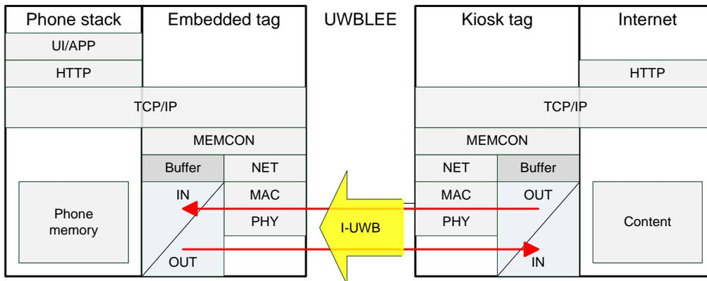
Figure 12. Schematic layout of the communication system when a mobile phone connects to the Internet via a memory-tag-based Internet kiosk.
