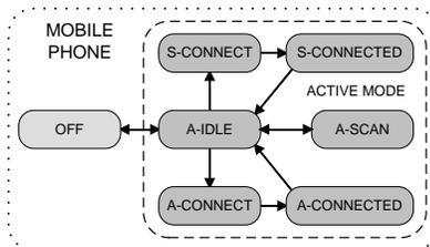
Figure 5. Active (and semi-passive) UWBLEEE MAC states on a mobile phone. Active states denoted with A, semi-passive with S.
