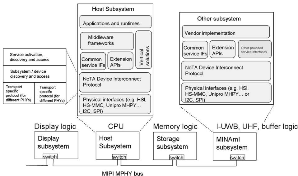
Figure 2. NoTA extension architecture for MINAmI subsystem, where HSI = High Speed Serial Interface; HS-MMC = High Speed MultiMediaCard; SPI = Serial Peripheral Interface bus.
