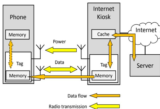
Figure 11. Mobile phone operating in passive or semi-passive mode to download data through an Internet Kiosk.
