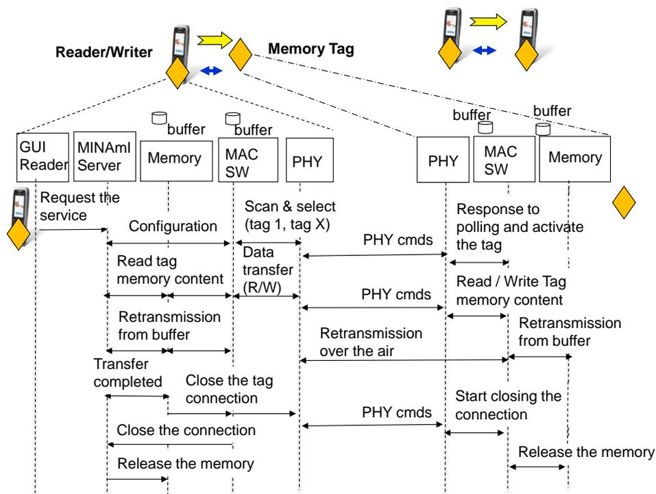
Figure 8. Basic MINAmI subsystem communication setup sequence
