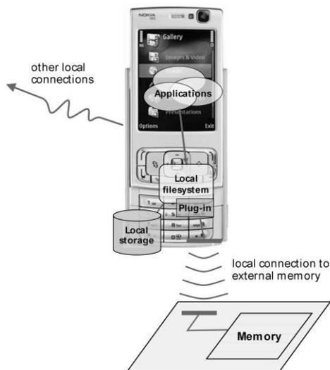
Figure 9. File system view of a mobile phone reading a passive memory tag: a cheap tag without its own processor [11].
