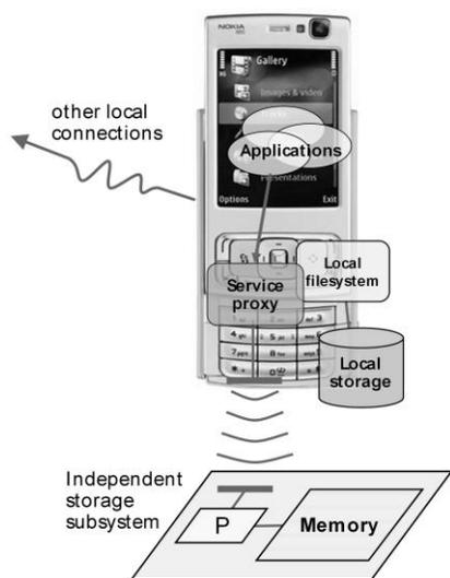
Figure 10. File system view of a mobile phone reading a passive memory: a more expensive tag with its own processor [11].
