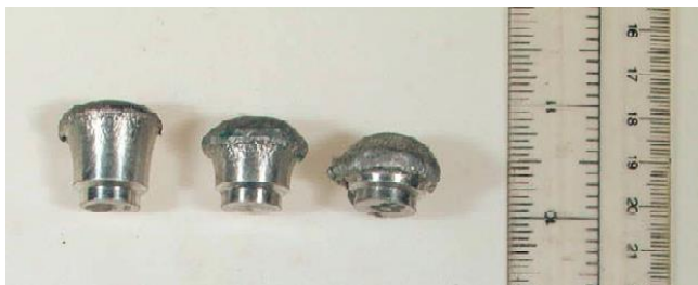
Figure 9. Deformed 6061-T6 aluminum projectiles after perforation 0.125, 0.25, and 0.5 inch thick (left-to- right) aluminum targets.
