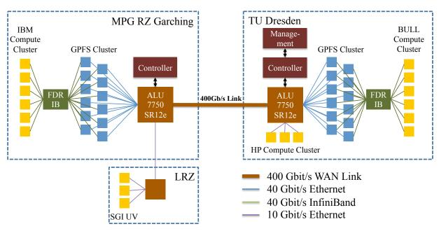
Figure 7: Overview 400-Gigabit/s-Testbed architecture
