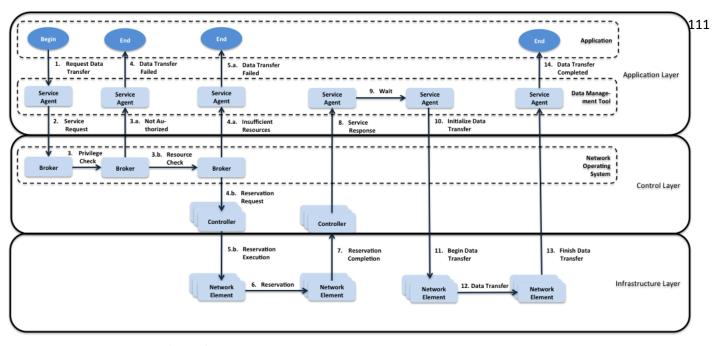
Figure 6: Integrated SDN communication process negotiating for network resources
