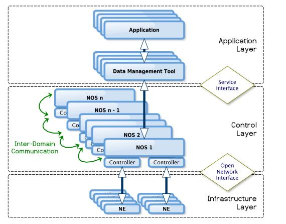
Figure 2: Integrated multi layer, multi domain SDN architecture
