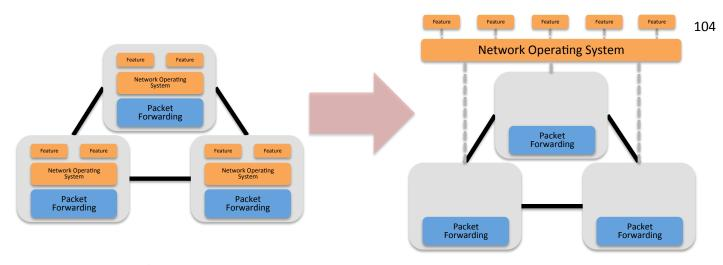
Figure 1: Conventional vs. SDN driven network, full separation of forwarding and control plane
