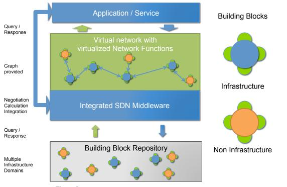
Figure 3: Functional model of an application-driven network architecture
