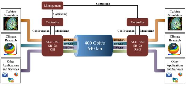
Figure 8: Setup of the Bandwidth-on-Demand Demonstrator
