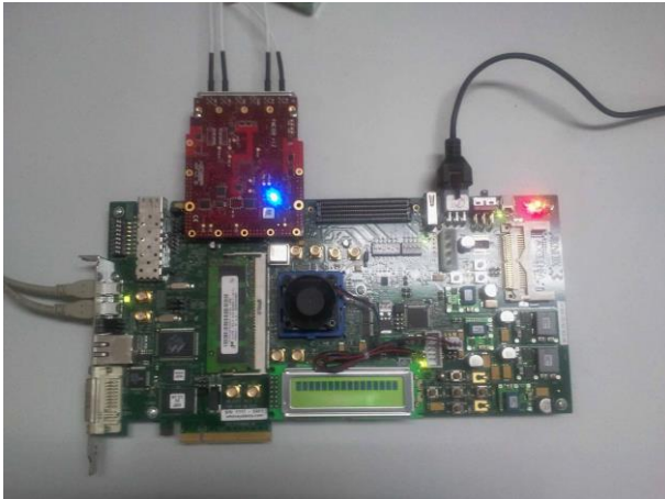
Figure 11. FPGA hardware platform setup
