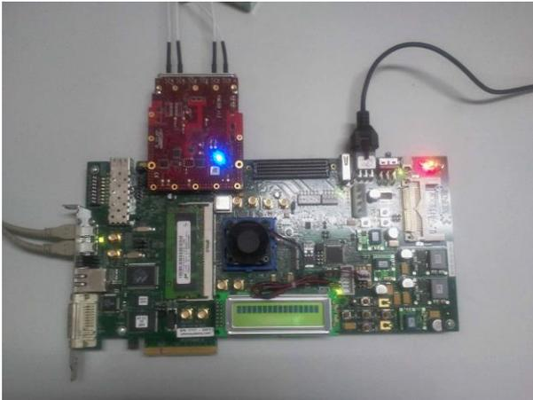
Figure 11. FPGA hardware platform setup
