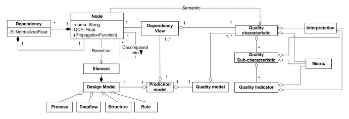
Figure 3. An overview of the elements of the prediction models, expressed as a UML class diagram
