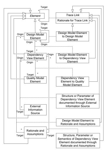
Figure 4. A meta model for trace-link information, expressed as a UML class diagram
