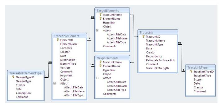
Figure 7. Entity-relationship diagram of the trace-link database of the prototype traceability tool
