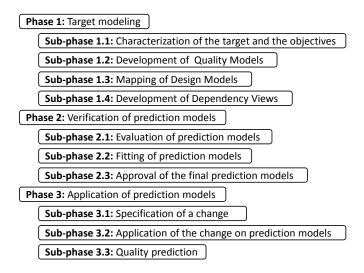
Figure 1. A simplified overview of the process of the PREDIQT method
