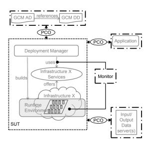
Figure 6. A test architecture for GCM-based deployment
