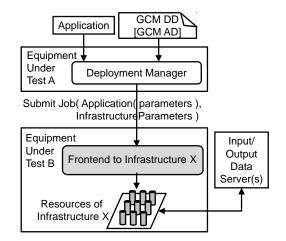
Figure 10. Single infrastructure with a bridge and I/O servers
