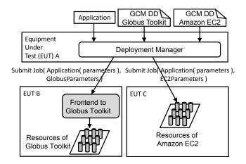
Figure 14. Test configuration "Two infrastructures and bridges" exemplified by Globus Toolkit and Amazon *Elastic Compute Cloud* (EC2)
