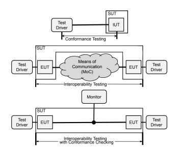
Figure 4. Three approaches to testing in standardization
