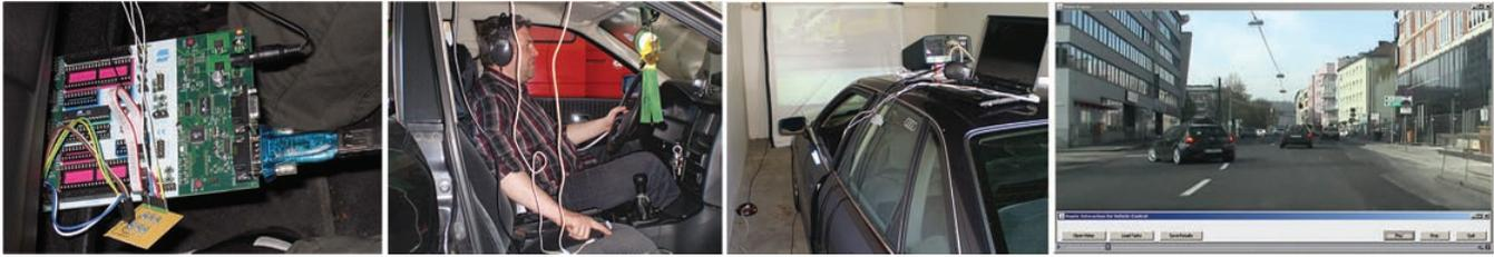
Figure 1. Experimental setting for the trace-driven experiment with vehicle control signals taped via Atmel  $\mu C$  and forwarded to the control application (leftmost image), screen shot of the prerecorded test run as shown the participants during the experiment (rightmost picture).
