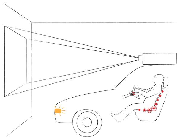
Figure 4. Scribble of the driving simulator setting as used for trace-driven simulation. The car was parked in a darkened garage with vehicle controls connected to a microcontroller. A video projector was used to generate a close-to-reality street view in the front shield.
