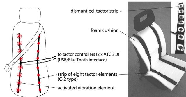
Figure 5. Vibro-tactile notifications were delivered via the driver seat. Therefore, two strips of eight voice coil transducers each were embedded into the seat. The foam cushion was applied to ensure comfortable sitting.
