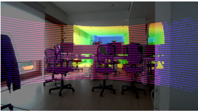
Figure 7. Point cloud reprojection onto RGB image, after intrinsic and extrinsic calibration.
