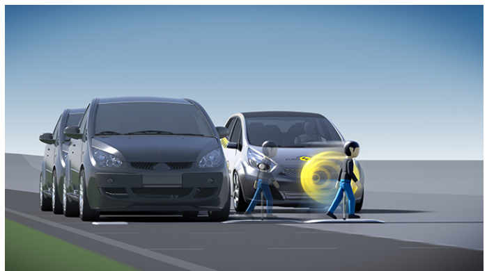
Fig. 2. Test setup for pedestrian detection, where a pedestrian (child as a dummy) crosses the road behind a parked car in a scenario for testing Automatic Emergency Braking (AEB) based on Euro NCAP regulations [25].
