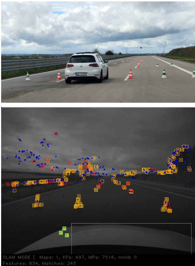
Fig. 6. Test area on the top of the figure with pylons and test vehicle as well as detected feature points using ORB-SLAM (rectangles) on the bottom.
