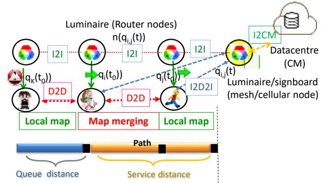
Figure 12. Graphical representation of the simultaneous localization and mapping problem using connectivity as a function of node density, mobility and transmission range.
