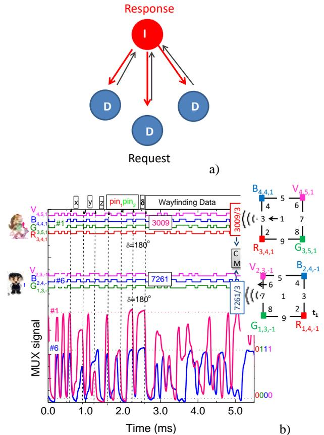
Figure 9. a) Communication channels established between the infrastructure and the vehicles for geolocation and navigation. b) MUX/DEMUX signals assigned requests from two users ("3009" and "7261") at different poses ( $C_{4,4,1}; \#1W$  and  $C_{2,3,-1}; \#6W$ ) and in successive instants ( $t_1$  and  $t_3$ ).
