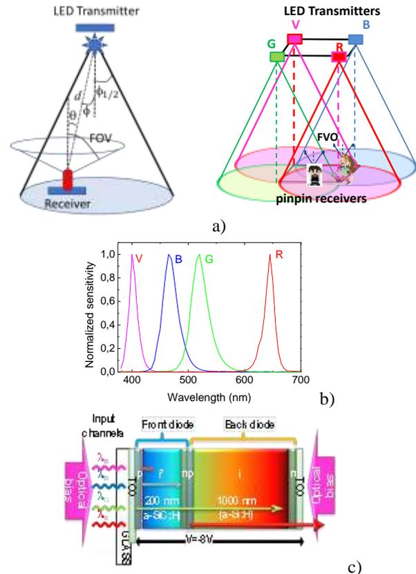
Figure 2. a)3D relative positions of the transmitters and receivers. b) Spectra of the input channels. c)Configuration and operation of the pin/pin Mux device
