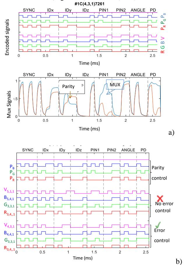
Figure 7. Encoding/decoding process with and without check parity error. a) Transmitted code signals [R G B V : P<sub>R</sub> P<sub>G</sub> P<sub>B</sub>] and received MUX and Parity signals. b) Decoded information with and without error control assigned to a request from user "7261" at cell  $C_{4,3,1}$  #1 NE.
