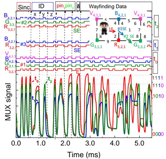
Figure 8. Fine-grained indoor localization and navigation in successive instants. On the top the transmitted channels packets are decoded [R, G, B, V]
