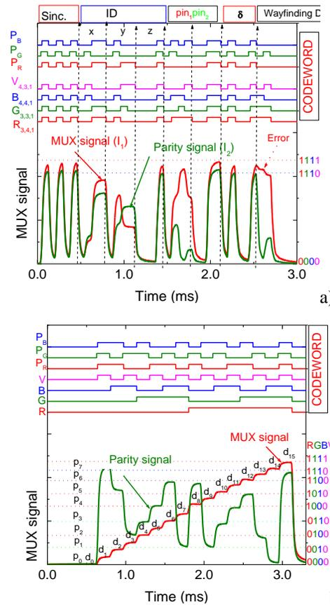
Figure 6. Code and parity MUX/DEMUX signals. On the top the transmitted channels [R G B V :  $P_R P_G P_B$ ] are shown. a) Calibrated cell. b) Error control assigned to a request from user "7261" at  $C_{4,3,1}$ ; #1 N.
