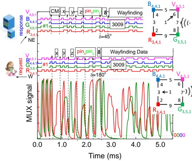
Figure 10. Request from user “3009” and response from the CM to him. On the top the transmitted channels packets are decoded [Xi,j,k].
