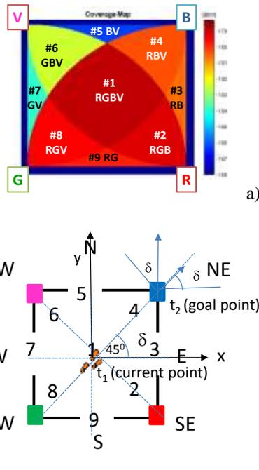
Figure 5. Illustration of the coverage map in the unit cell: a) Fingerprint regions (#1-#9). b) Steering angle codes (2-9).
