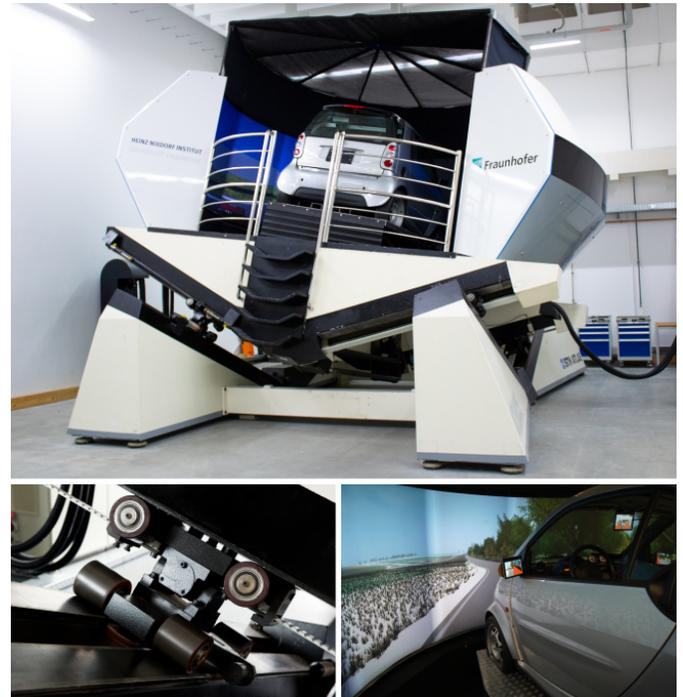
Figure 3. ATMOS Dynamic Driving Simulator.
