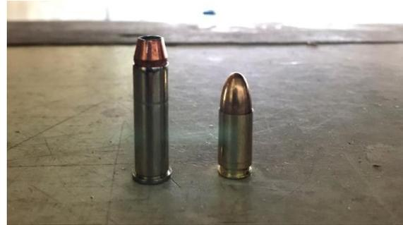
Figure 5. Left side: .357 Mag 158 Gr. Right side: 9 mm Luger 124 Gr.
