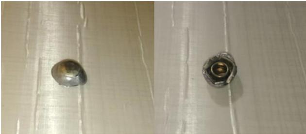
Figure 11. Deformed projectile of test number 12M.
