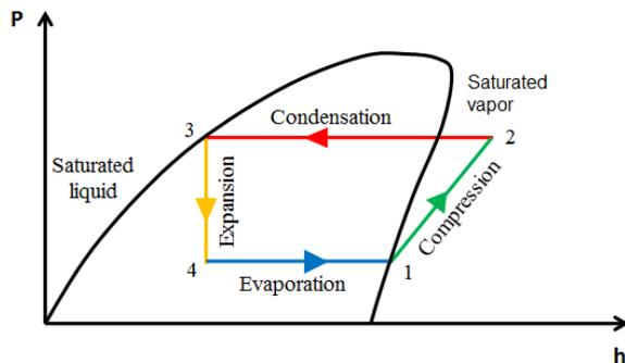
Figure 2. Diagram pressure (p) vs enthalpy (h) [22].
