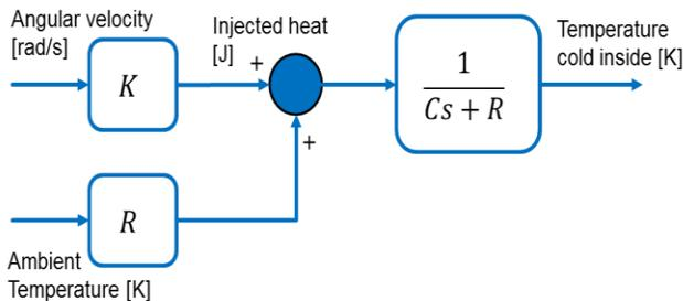
Figure 4. Linearized model dependent on the speed of the compressor [1].
