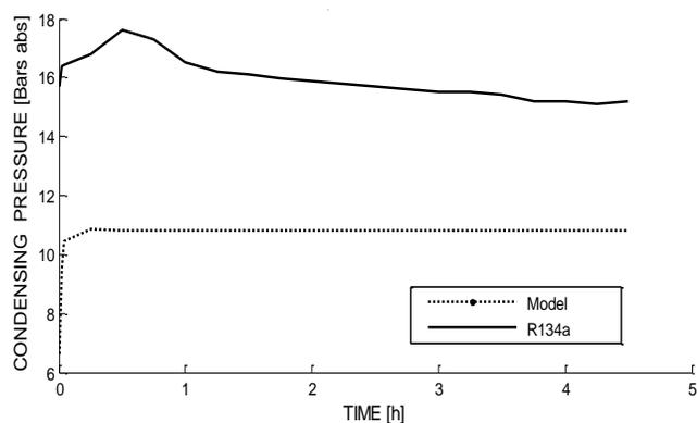
Figure 14. Behavior of the pressure in the condenser.
