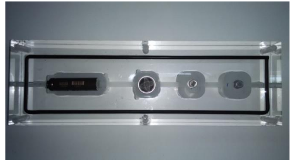
Figure 11. Custom-designed methacrylate box to host the gas sensors.
