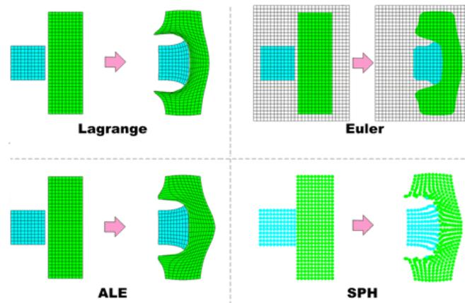
Figure 4. Examples of Lagrange, Euler, ALE, and SPH simulations on an impact problem [14].
