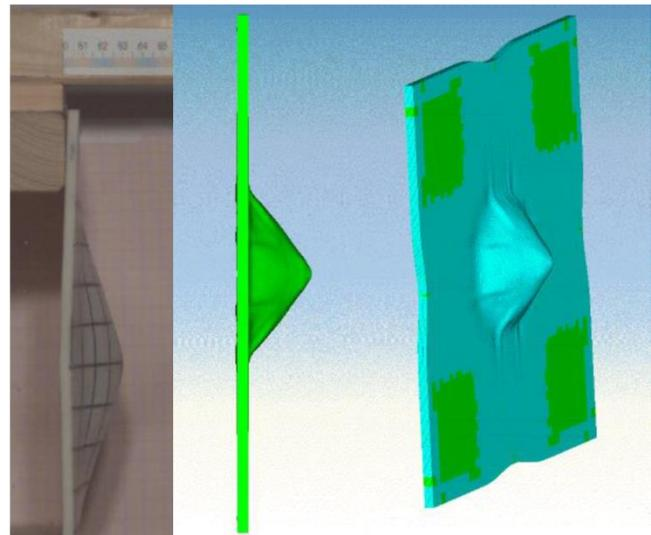
Figure 17. Effect of a 5.5 mm target impact by a 9×19 mm Parabellum bullet at 348 m/s.
