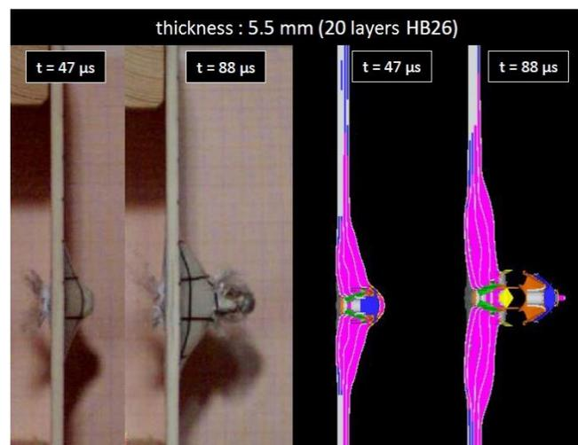
Figure 14. Effect of a 5.5 mm target impact by a 7.62×39 mm bullet at 686 m/s, 47 μs and 88 μs after the initial impact.
