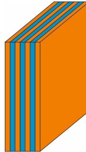
Figure 13. Geometry of a target plate: alternating layers of fibers and matrix are used in the computer model.
