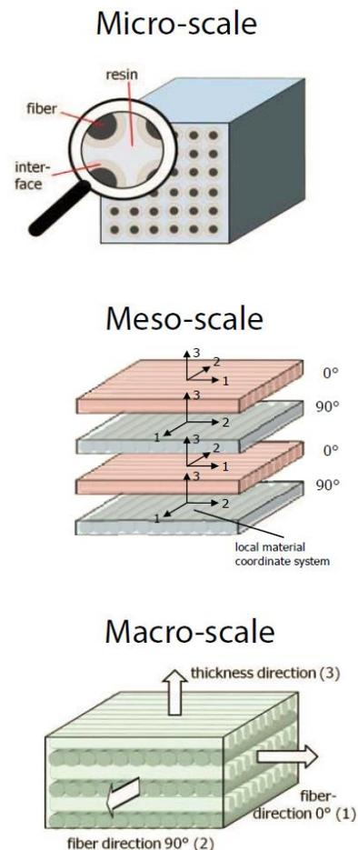
Figure 11. Micro, meso and macro mechanical model of fiber reinforced composites [27].
