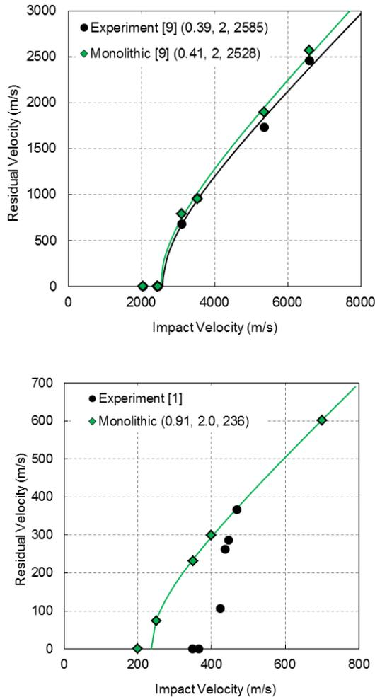
Figure 8. Experimental and numerical impact residual velocity results for impact of 6 mm diameter aluminum spheres against 15 kg/m<sup>2</sup> Dyneema® HB26 at normal incidence (left) and impact of 20 mm FSP against 10 mm thick HB26 at normal incidence (right).
