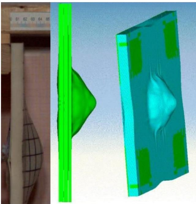
Figure 16. Effect of a 16.2 mm target impact by a 7.62×39 mm bullet at 679 m/s.
