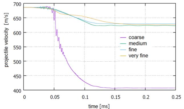
Figure 20. Convergence analysis: comparison of the projectile velocity (7.62×39 mm bullet) at different mesh sizes.
