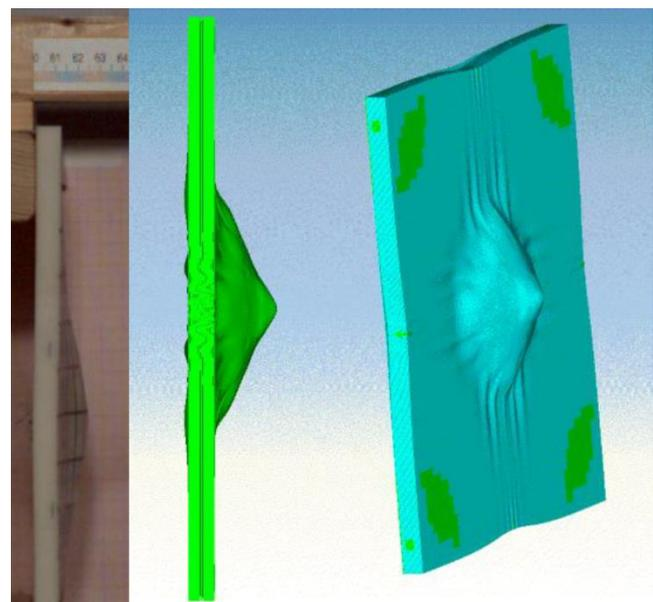
Figure 18. Effect of a 11.0 mm target impact by a 9×19 mm Parabellum bullet at 343 m/s.
