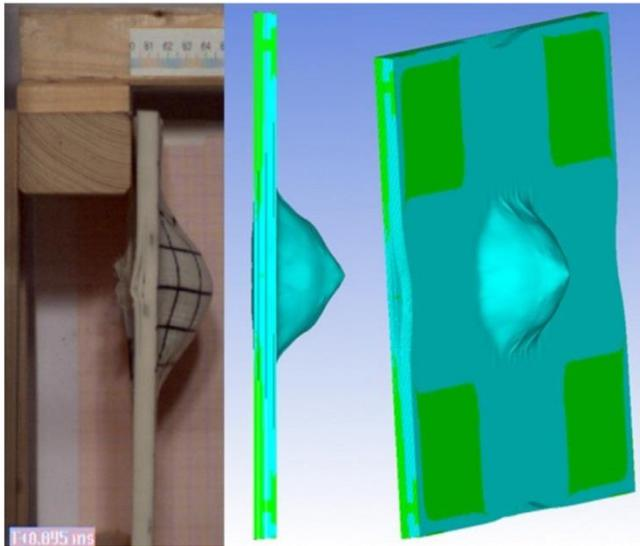
Figure 15. Effect of a 11.0 mm target impact by a 7.62×39 mm bullet at 682 m/s.
