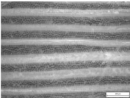
Figure 12. Cross section of a Dyneema® HB26 panel.
