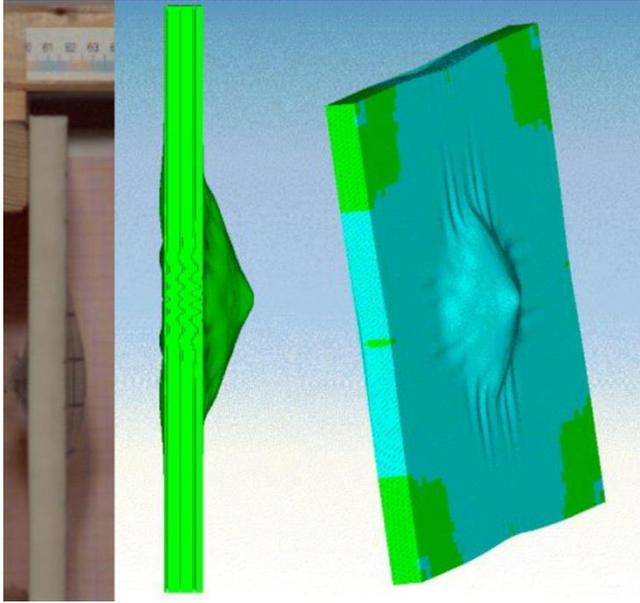
Figure 19. Effect of a 16.2 mm target impact by a 9×19 mm Parabellum bullet at 346 m/s.
