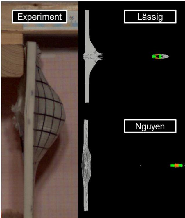
Figure 10. Bulge of a 11 mm target impact by a 7.62×39 mm FMJ projectile at 689 m/s (experiment) and the simulation results using both “state-of-the-art” models of Lässig and Nguyen 700 m/s.
