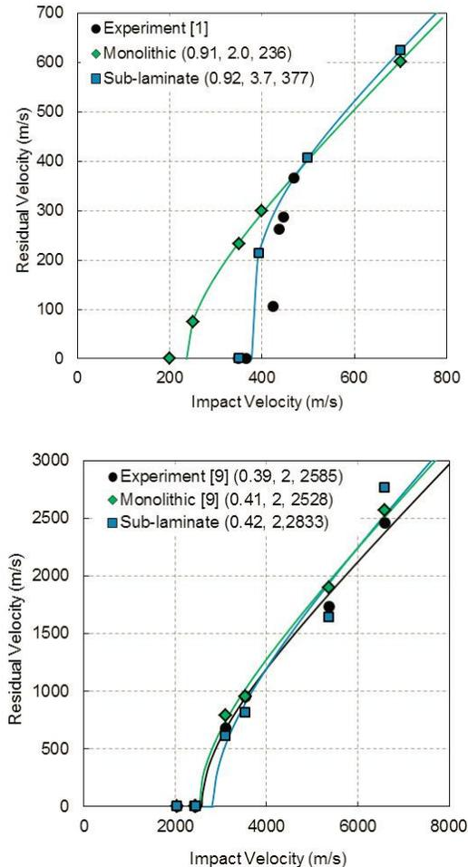
Figure 9. Comparison of the experimental results with the two numerical models for impact of 20 mm FSP against 10 mm thick Dyneema® HB26 at normal incidence (left), and impact of 6 mm diameter aluminium spheres against 15 kg/m<sup>2</sup> HB26 at normal incidence (right).
