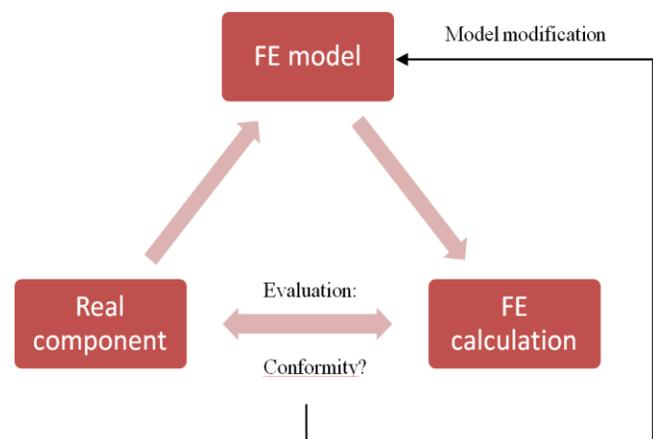
Figure 5. Basically iterative procedure of a FE analysis [15].
