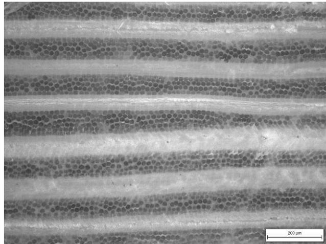
Figure 14. Cross section of a Dyneema® HB26 panel.
