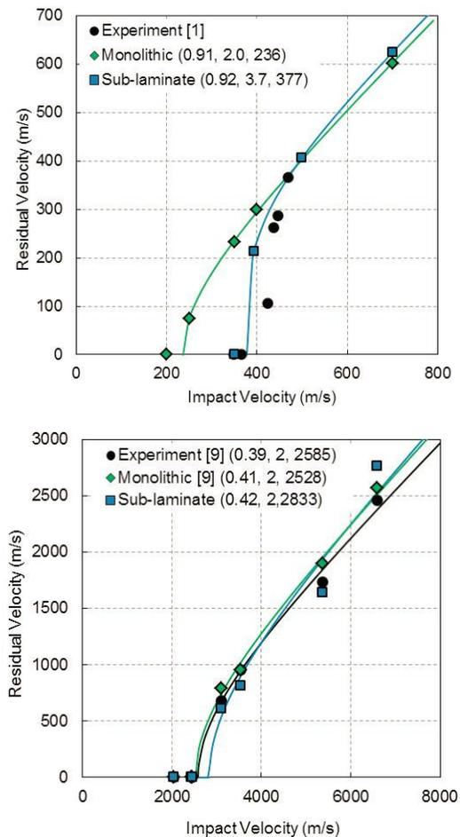
Figure 10. Comparison of the experimental results with the two numerical models for impact of 20 mm fragment simulating projectiles against 10 mm thick Dyneema HB26<sup>®</sup> at normal incidence (left), and impact of 6 mm diameter aluminium spheres against 15 kg/m<sup>2</sup> Dyneema<sup>®</sup> HB26 at normal incidence (right). Lambert-Jonas parameters (a, p, Vbl) are provided in the legend.
