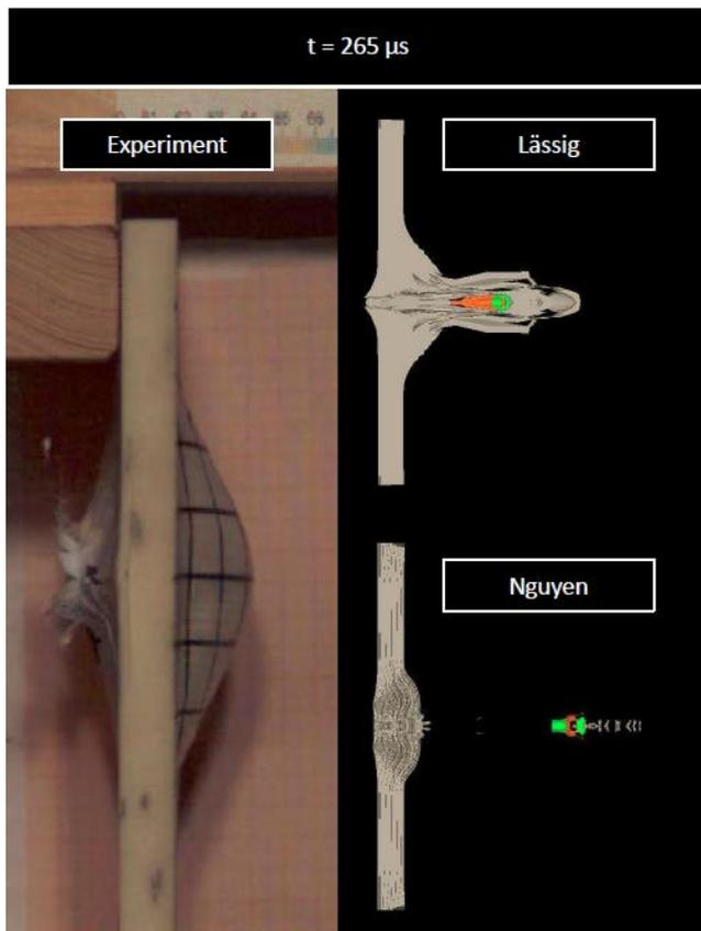
Figure 12. Comparing experimental results with the previous simulation models of Lässig [8] and Nguyen [9], 265  $\mu$ s after impact (grey = plastic deformation, green = elastic deformation, orange = material failure); projectile velocity: 674 m/s; target thickness: 16.2 mm (60 layers of HB26).
