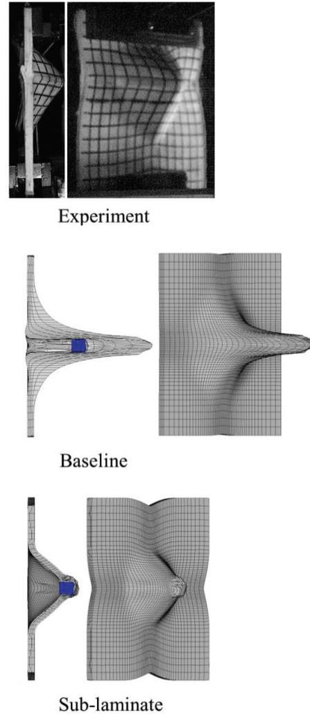
Figure 11. Bulge of a 10 mm target impact by a 20 mm FSP at 365 m/s (experiment) and 350 m/s (simulations), 400  $\mu$ s after the initial impact.
