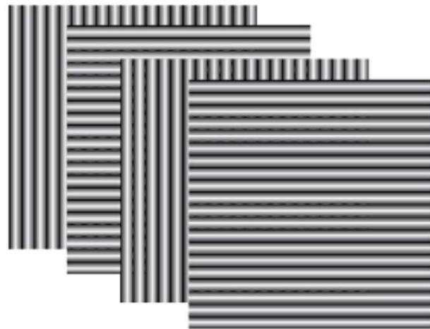
Figure 15. Setup / structure of a Dyneema® HB26 prepreg.
