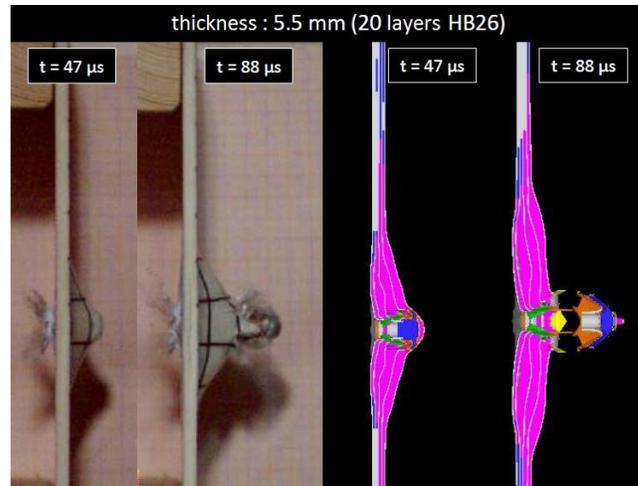
Figure 13. Effect of a 5.5 mm target impact by a 7.62×39 mm bullet at 686 m/s, 47  $\mu$ s and 88  $\mu$ s after the initial impact.
