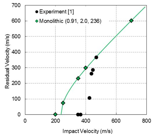
Figure 9. Experimental and numerical impact residual velocity results for impact of 6 mm diameter aluminum spheres against 15 kg/m<sup>2</sup> Dyneema<sup>®</sup> HB26 at normal incidence (left) and impact of 20 mm fragment simulating projectiles against 10 mm thick Dyneema<sup>®</sup> HB26 at normal incidence (right). Lambert-Jonas parameters ( $a$ ,  $p$ ,  $V_b$ ) are provided in the legend.
