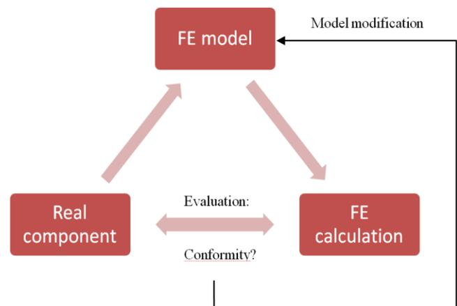
Figure 3. Basically iterative procedure of a FE analysis [15].
