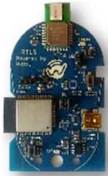
Figure 4. Wearable device prototype of the GuideMe project.
