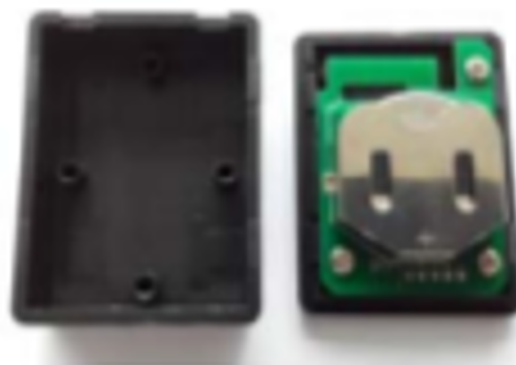
Figure 7. BLE node used in this work, a W901 wellcore module
