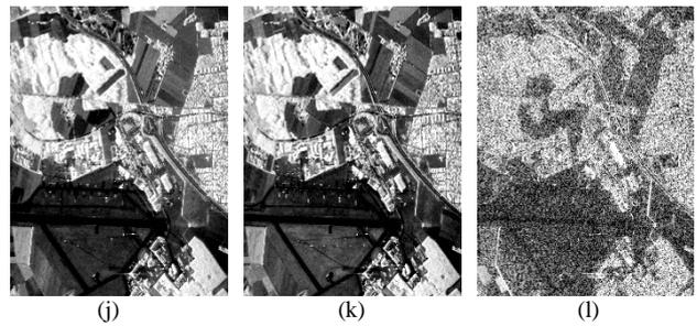
Fig. 3. (a) Original image. (b) Power spectrum image. (c) Bragg scattering for Cloud Decomposition. (d) Dihedral scattering. (e) Volume scattering. (f) Dbl scattering component (g) Hlx scattering component (h) Odd scattering component (i) Vol scattering component (j)  $K_d$  dihedral angular scattering component (k)  $K_h$  helix scattering component (l)  $K_s$  spherical scattering component
