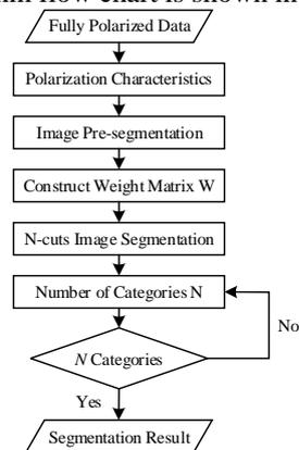
Fig. 2. Flow chart of region-based N-cuts algorithm
