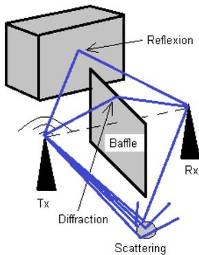
Figure 2. Multipath propagation
