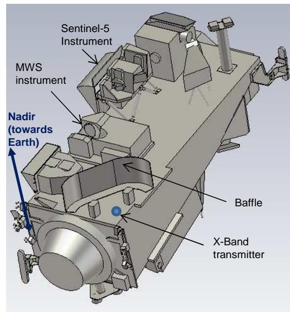
Figure 1. Model of “Satellite A” being part of MetOp Second Generation: Exemplary transmitter and instrument receiver positions
