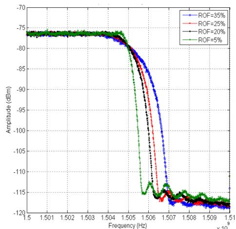
Figure 4. Sharper roll-off signal characterization: frequency response
