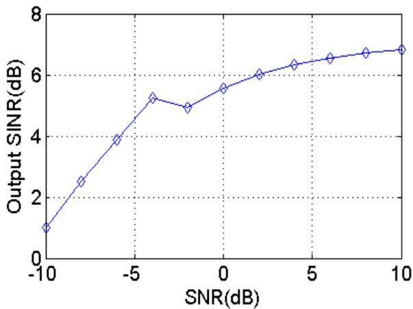
Figure 9. Output SINR per ISR for ISR = 3 dB
