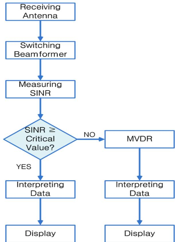
Figure 4. Flow chart of the hybrid TPMS beamformer
